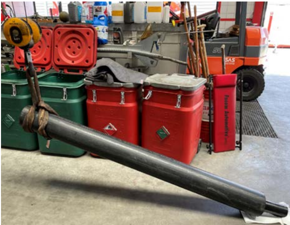
Fig. 6 set-up for slope test to determine the COF
